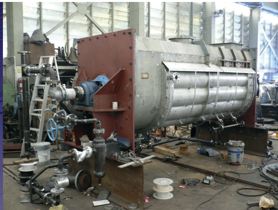
Pre-heater with bulb jacket
